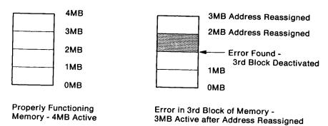
Figure 3-6. Memory Error Address Reassignment
